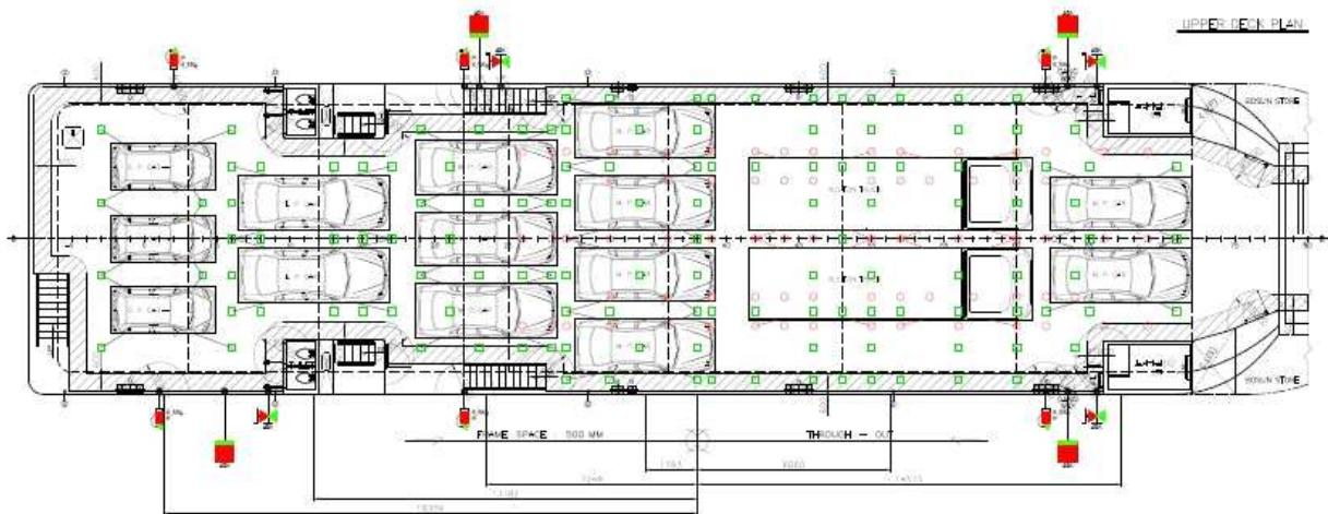
**F. 11.5 TON CARGO TRUCK LOADING CONDITION**
